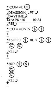
Before finishing a command string the user exits to perform a monitor command.
